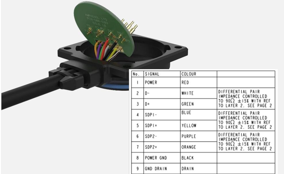
MOVE THE SHORTER, RED AND BLACK CORES OUT OF THE WAY OF THE PCB, DO NOT SOLDER THESE YET
